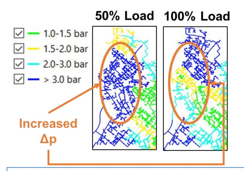
In low load scenarios the heat coming from TENT-A serves an even larger portion of Dunav's system, allowing a decrease in  $\Delta p$  at the plant, without reaching critical conditions at the peripheral sections of the network
