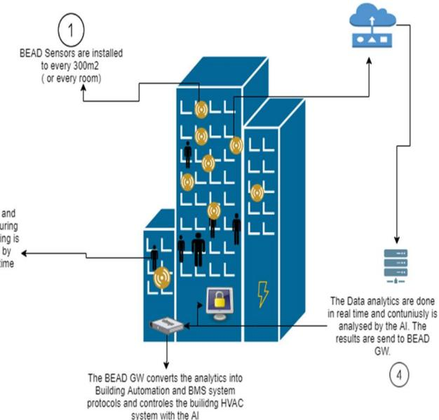
The BEAD Sensors are sending real time data of six different metrics to the Cloud based BEAD AI.
